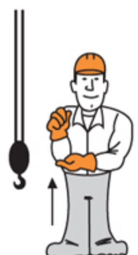
Use Auxiliary Hoist
