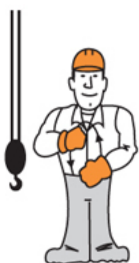
Crawler Crane Travel Both Tracks
