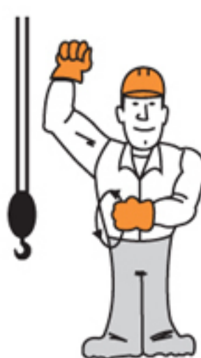
Crawler Crane Travel One Track
